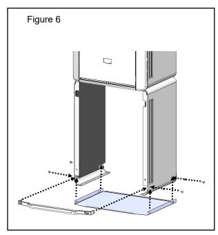
5. Place the bottom plate insulation panel onto the bottom plate (apply panel in either front-facing direction) (Figure 7).
