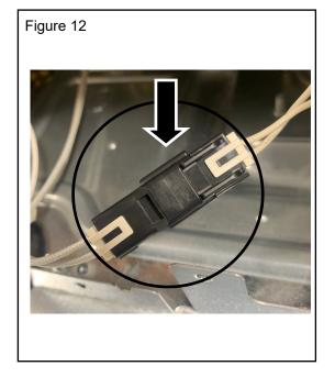
12. Disconnect and separate the green ceramic heater harness connectors (Figure 14).
